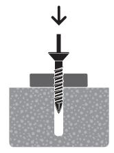
Install with either a socket hex driver or cordless impact driver. Apply pressure against the fixing and rotate to engage the first thread.
