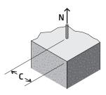
To achieve published tension loads the anchors should be installed at least 8 x the anchor drill diameter from a concrete edge. If edge distance is closer than 8 x the anchor drill diameter apply the appropriate reduction factor as outlined in the EDGE DISTANCE TENSION TABLE to the published load to ascertain the reduced load.
