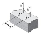
To achieve published tension and shear loads the anchors should be installed at least 12 x the anchor drill diameter between each other. If spacing between anchors is closer than 12 x the anchor drill diameter apply appropriate reduction factor as outlined in the SPACING TABLE to the published load to ascertain the reduced load.
