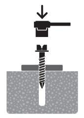
Install with either a socket or cordless impact driver. Apply pressure against the fixing and rotate to engage the first thread.
