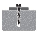
Continue to tighten the anchor until hex head is firmly seated against fixture. Installation complete!
