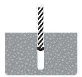
With the correct diameter drill bit, drill a hole to the depth of at least one diameter of the anchor deeper than required embedment.
